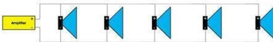
3. It is normal practice to wire out from the amplifier to the 1<sup>st</sup> or nearest speaker, and then on to any subsequent speakers. Looping in and out is best practice, although if you need to wire off to an existing circuit, teeing off is perfectly acceptable.
